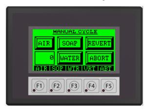
P. Press Soap (or F2) to begin the Soap (Detergent/Water mix) spray into the Cylinder. When in Manual Mode, each selection is a toggle switch either ON or OFF. Press Soap or F2 to turn on and off the Soap Injection.
